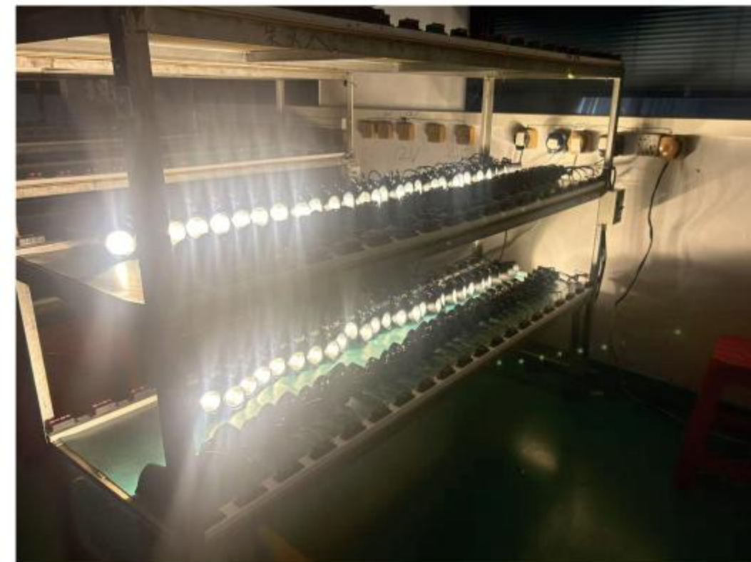
Aging test area
